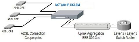
Figure 2-3 NCT480 Link Aggregation Illustrate
